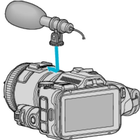
2 Open the cover of the microphone connector and connect the cable of the external microphone.
